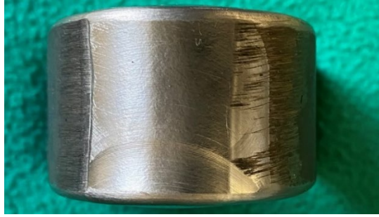
Figure 6. Specimen with grinded sharp edge after bend test
