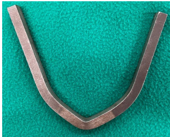
Figure 7. Example of "peaking" specimen
